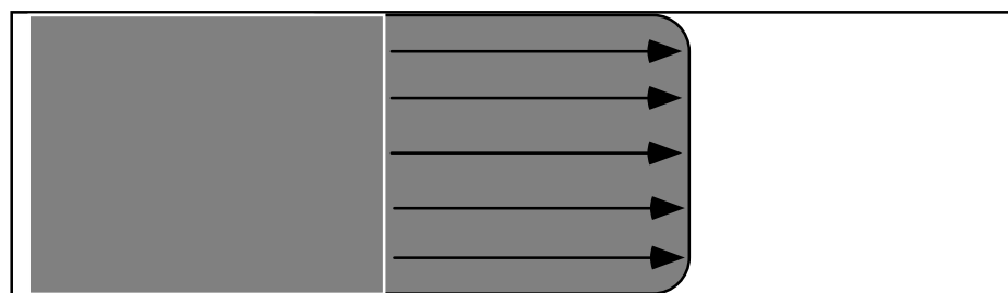
Bulk Flow arising from an Electroosmotically-driven system.
